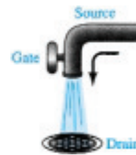
Figure 5.3 Water analogy for the JFET control mechanism.
