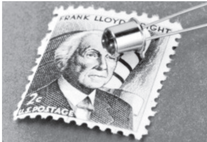
Figure 20.34 RCA IR-emitting diode: (a) construction; (b) photo; (c) symbol. (Courtesy RCA Solid State Division.)
