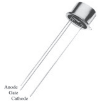
Figure 21.22 Typical GTO and its terminal identification. (Courtesy General Electric Company.)
